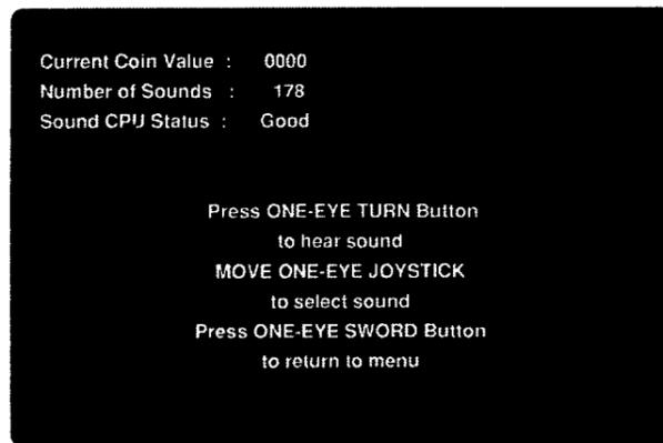
Figure 2-5 Sound Board Test Screen
