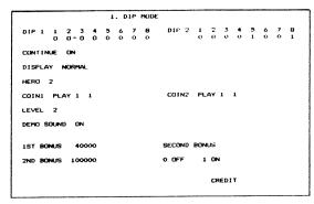
Set up the Dip-Switch settings as per the Table in Figure 3. The screen displays each bit as a `1' or `0' (on or off).
