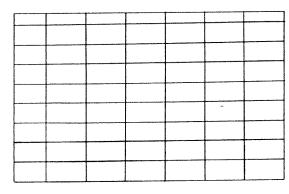
Adjust monitor for a square pattern throughout the display and on the edge of the monitor.
