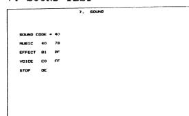
Set up the Sound Code (?) to 41-7B or 81-BB by moving the joystick, or by pressing the Kick Button at CO-FF.
