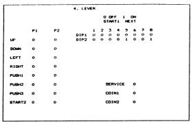
When a joystick or button is activated, the 'O' on the display will turn to a '1'.
