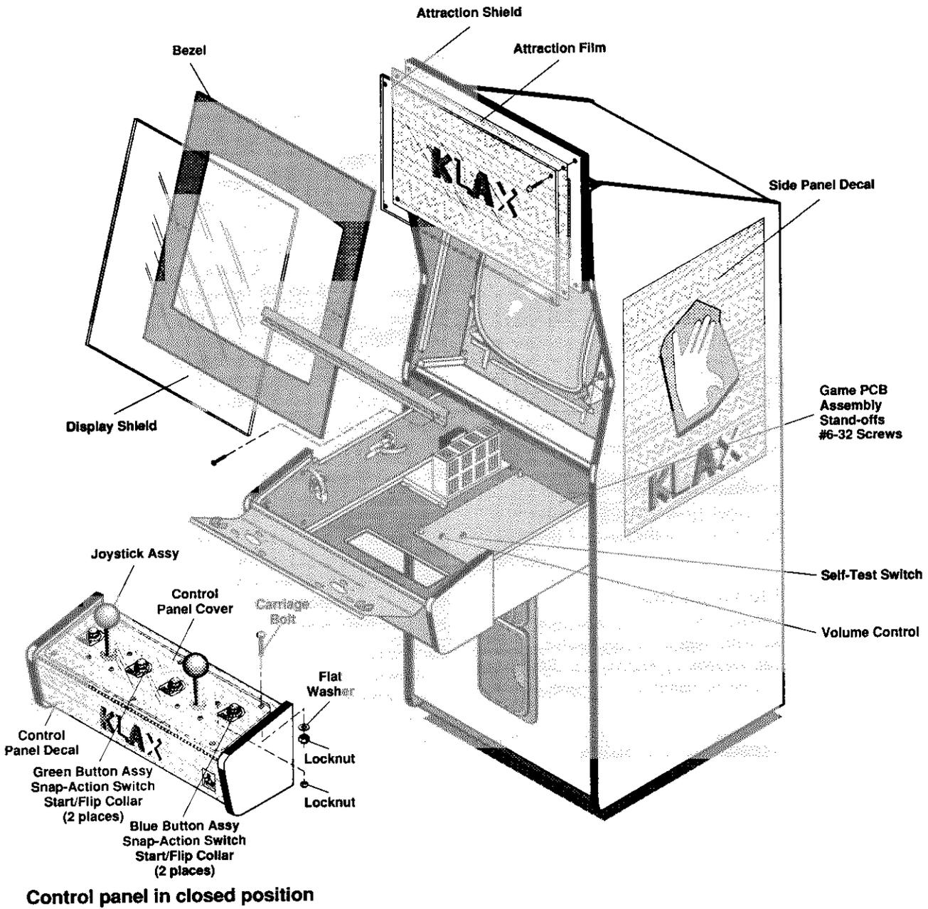
**Figure 1-2 Klax Kit Parts Installed in a Cabinet**
