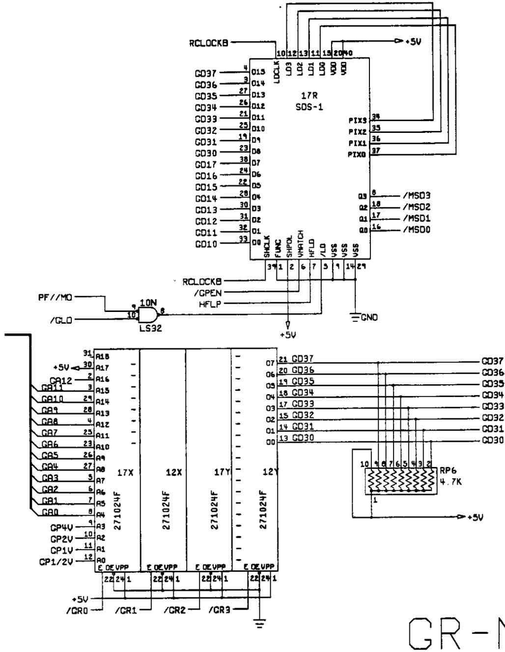
Figure 5-1 Klax Game PCB Assembly Schematic Diagram, Sheet 7 of 9
