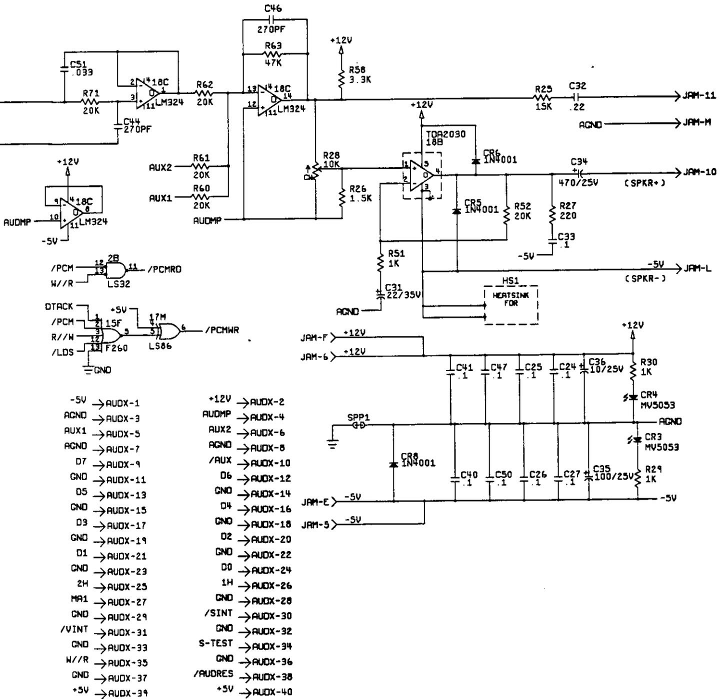
Figure 5-1 Klax Game PCB Assembly Schematic Diagram, Sheet 4 of 9
