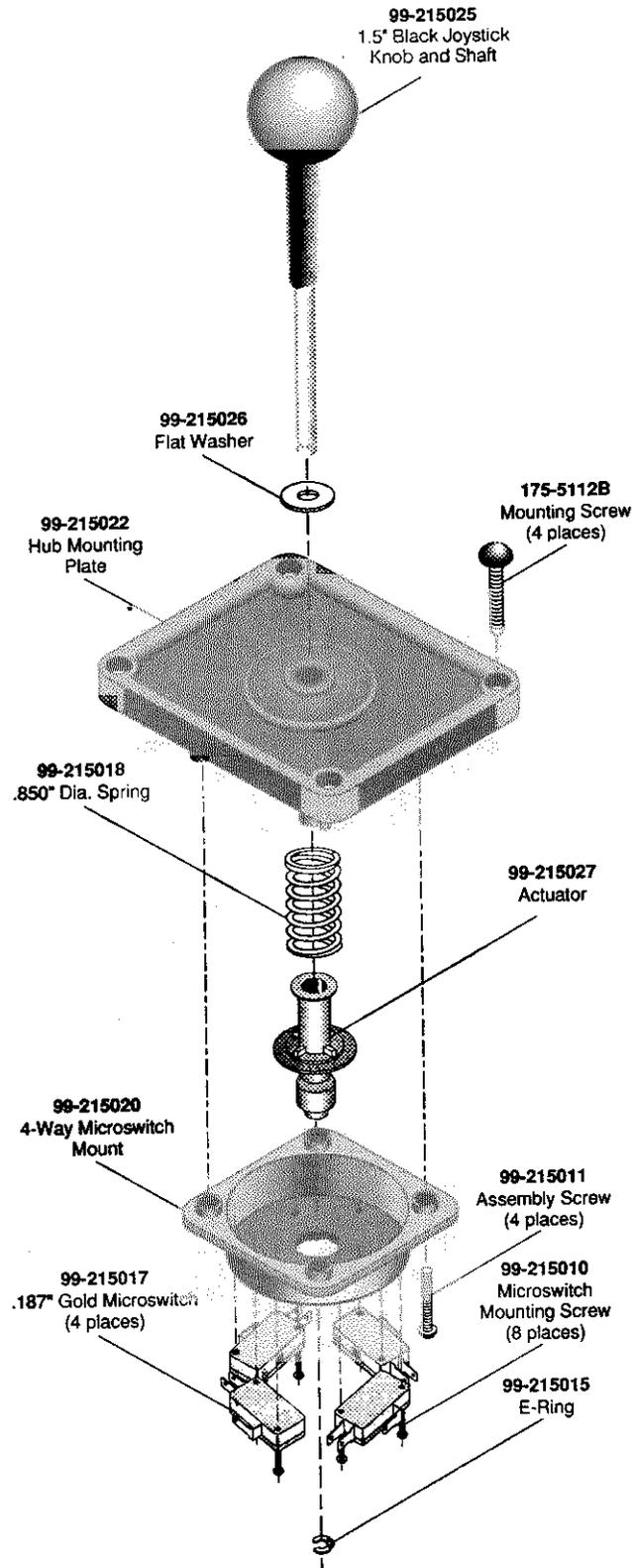
**Figure 4-2 Joystick Assembly**
