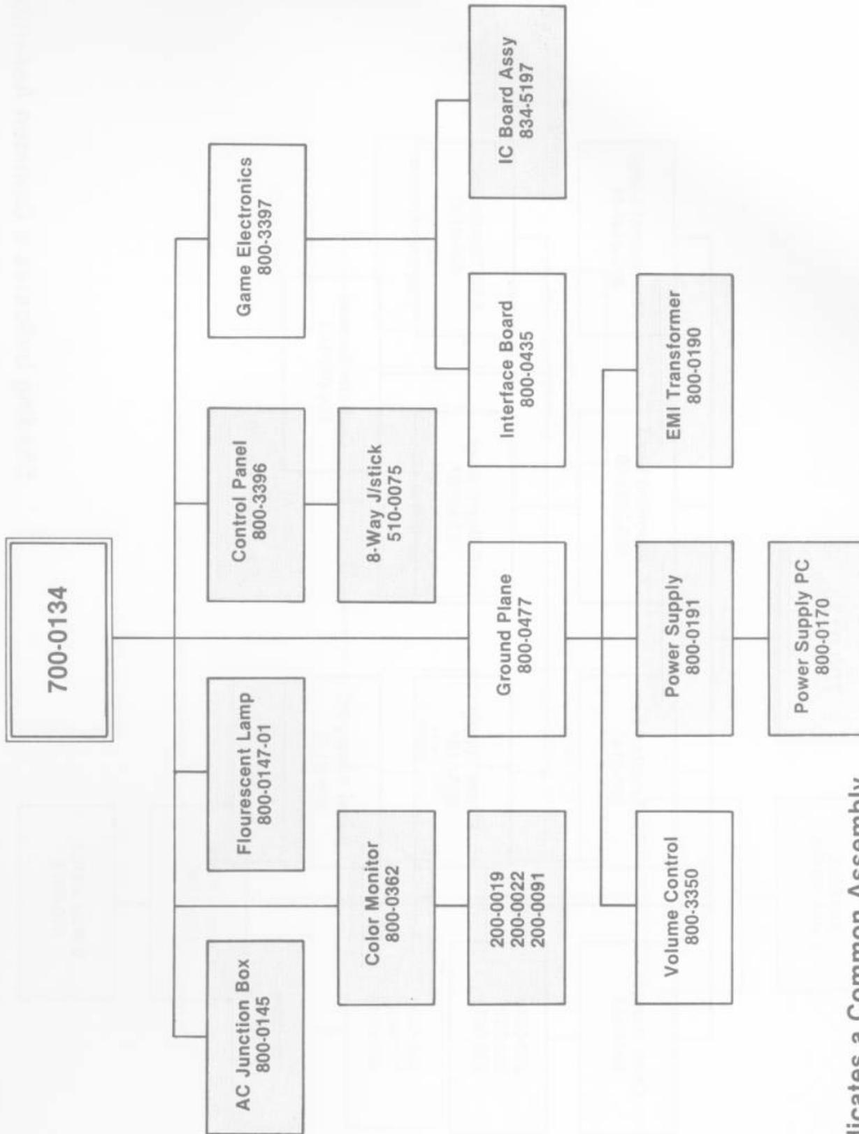
Shading indicates a Common Assembly
